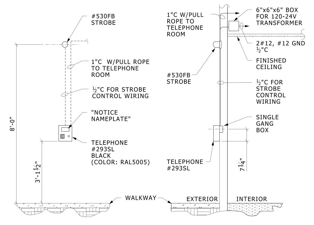
SEE DETAIL #1675005 FOR WIRING SEE DETAIL #1675006 FOR DRILLING DETAIL ON TELEPHONE
